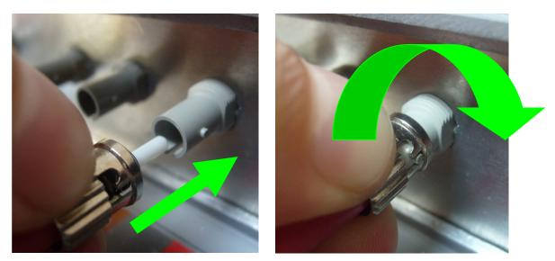
**5.2.4.** Secure the fiber optic bundle strain relief to the transducer housing. Make sure all of the individual fiber optic cables have a smooth bend radius. The fiber optics can be damaged if bent too tightly. Fold the protective tape over the fiber optic cables.
