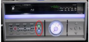
Plug in the AUX Components on the side of the CinemaVision Controller.
