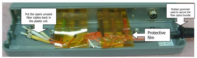
**5.2.5.** Connect the Power Supply cable to the Transducer. Route the cable to one of the round notches near where the fiber optic bundle exits the housing.
