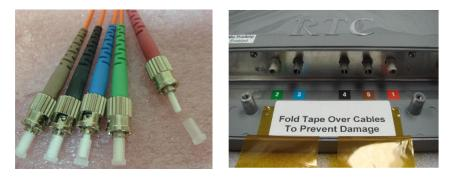
**5.2.3.** Remove the dust caps on all the fiber optic connectors on the transducer. Matching the fiber optic connector colors with the labels on the transducer, align the ridge on the cable connector with the notch of the transducer's connector. Insert the fiber optic cable connector until fully seated, then gently turn the ring clockwise until it stops (approximately one quarter turn). Perform the same procedure on the remaining fiber optic cables.
