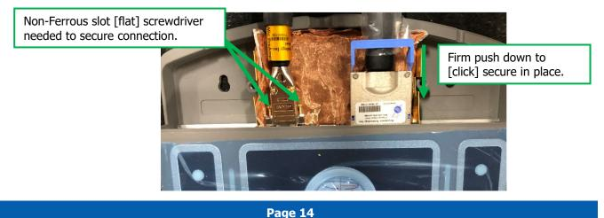
**5.2.9.** Carefully to install the shielding pillow in place when closing the top cover and making sure to align all cables with their respective exit notches in the housing. Best practice is to insert the top at an angle so you can feel if the pillow casing is not caught in the Transducer top mounting hole. After sitting the transducer top flush while the housing hand crank the black thumb screws to hold the top in place.
