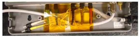
**5.2.6.** Carefully pull up the preinstalled protective cable cover film over these connections, making sure not to pinch any of the cables under the screw posts.
