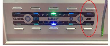
Plug in the AUX Components on the side of the CinemaVision Controller. AUX Input is HDMI connection.
