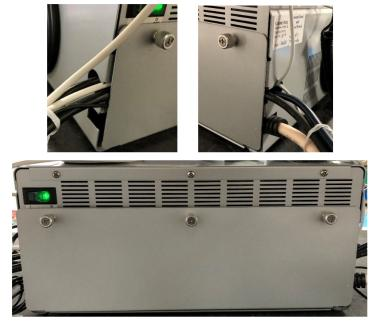
**5.3.13.** Install the rear cable cover once all functions verified to be working.
